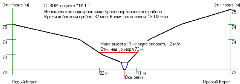
Figure 1: Site №1 – the removal from hydraulic unit makes 0,95 km.
