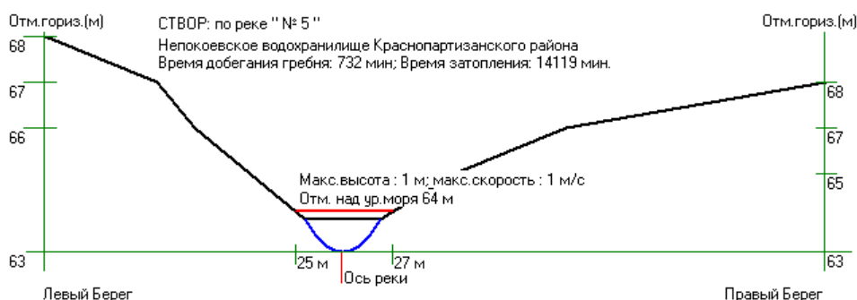
Figure 5: Site №5 – the removal from hydraulic unit makes 15,7 km.
